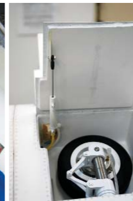
This is looking into the lower fuselage area, near the nose gear retract. Air tanks to each side, color coded air lines to track down a leak should it happen. Right: The main gear wheel well is pretty large. There is plenty of clearance to mount the door cylinders and route their air hoses.
